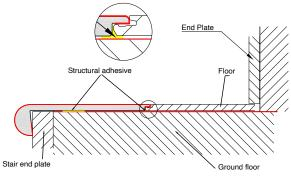
5mm Flush stair nose are suitable for 5mm floor, 7mm Flush stair nose are suitable for 7mm floor, the thickness of the floor and the thickness of the stairs at 0.5mm difference can be leveled by glue, when the thickness difference exceeds 0.5mm, you can use hard gasket leveling.
